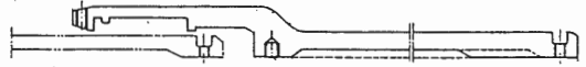
図6 P III 受挿連絡管 Fig. 6 Connecting piece with socket and spigot (P II - P III)
