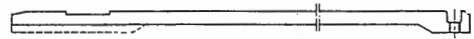
図7 P II - P III 両挿連絡管 Fig. 7 Connecting piece with double spigot (P II - P III)
