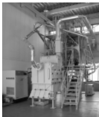
RCP (Roll Compaction Process) facility for quasi-mass production of magnesium alloy
