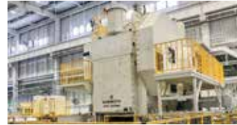
C2F-20GWL mechanical press for forging at the production line of CVJ (constant velocity joint) for cars (JTEKT Tadomisaki Plant)
