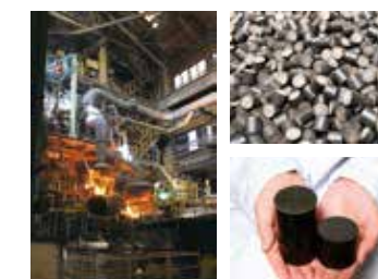
A cupola using bio-coke (right)
